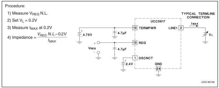
Figure 1. Termline Impedance Measurement Circuit
