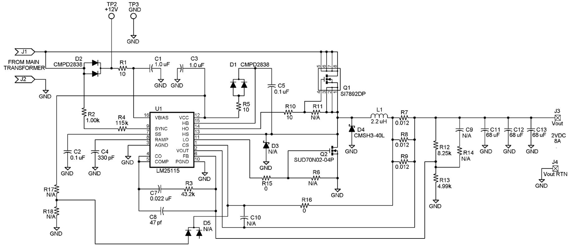
(Inputs from LM5025 Forward Active Clamp Converter, 36V to 78V)
