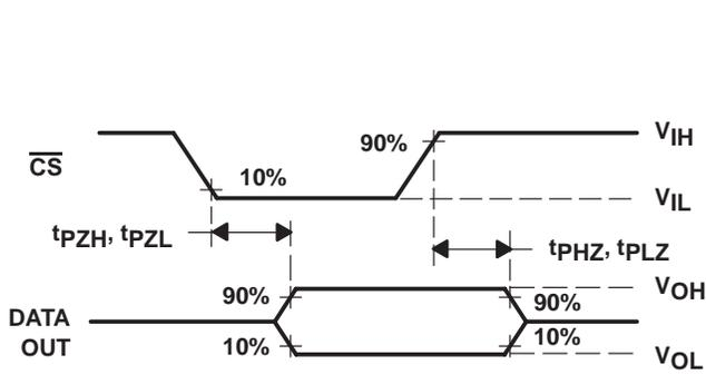
**Figure 8. DATA OUT to Hi-Z Voltage Waveforms**
