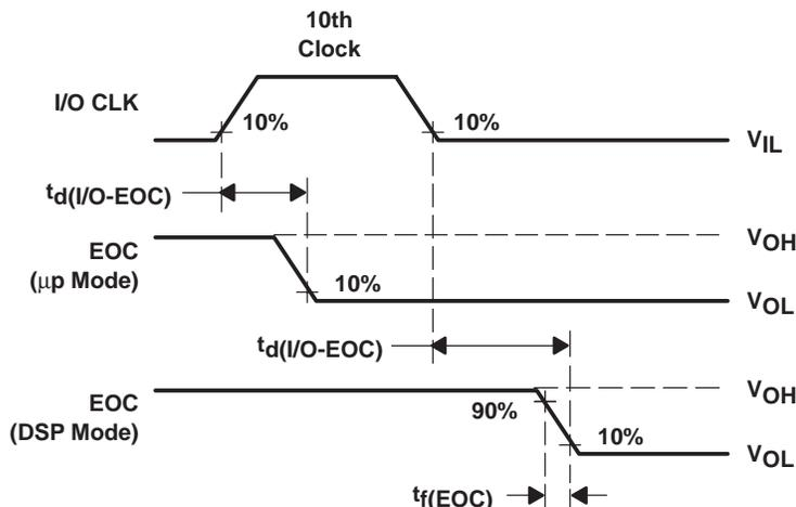
Figure 13. I/O CLK and EOC Voltage Waveforms
