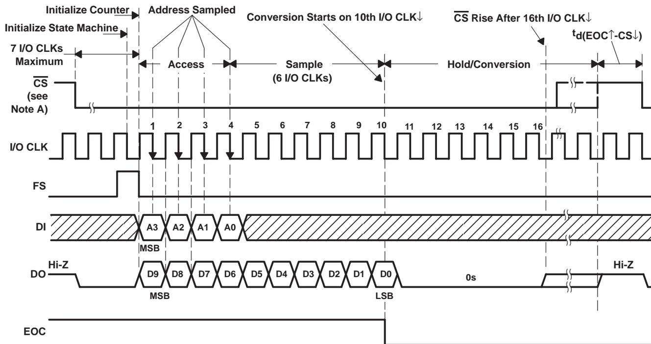
NOTE A: To minimize errors caused by noise at  $\overline{CS}$ , the internal circuitry waits for a setup time after  $\overline{CS} \downarrow$  before responding to control input signals. No attempt should be made to clock in input data until the minimum  $\overline{CS}$  setup time elapses.
