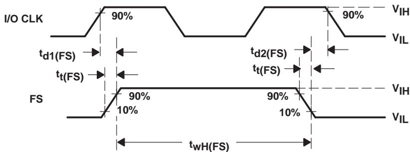
Figure 14. FS and I/O CLK Voltage Waveforms
