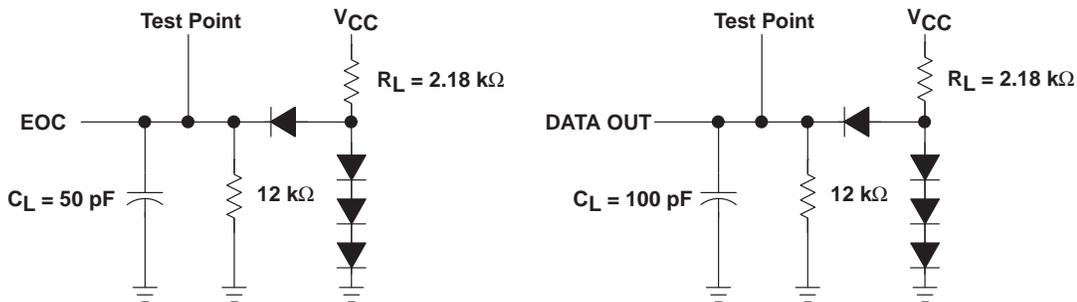
Figure 7. Load Circuits
