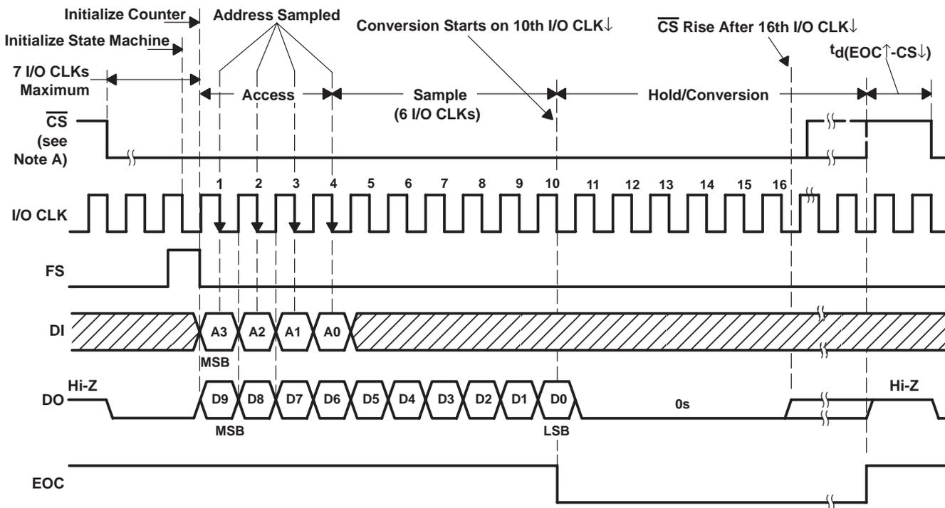
NOTE A: To minimize errors caused by noise at  $\overline{\text{CS}}$ , the internal circuitry waits for a setup time after  $\overline{\text{CS}}\downarrow$  before responding to control input signals. No attempt should be made to clock in input data until the minimum  $\overline{\text{CS}}$  setup time elapses.
