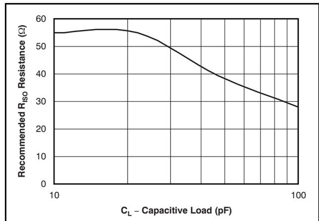
Figure 43. Recommended R<sub>ISO</sub> vs Capacitive Load
