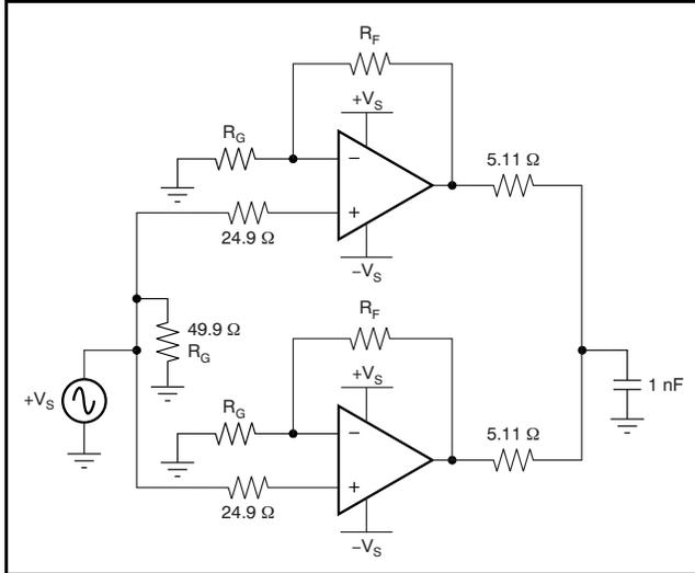
Figure 48. Parallel Amplifiers for Higher Output Drive
