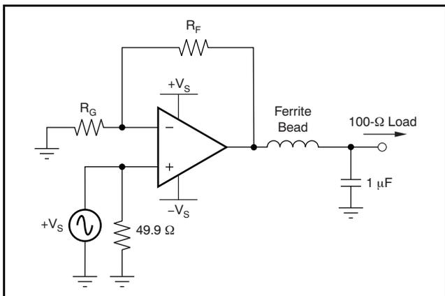
Figure 45. Ferrite Bead to Isolate Capacitive Load
