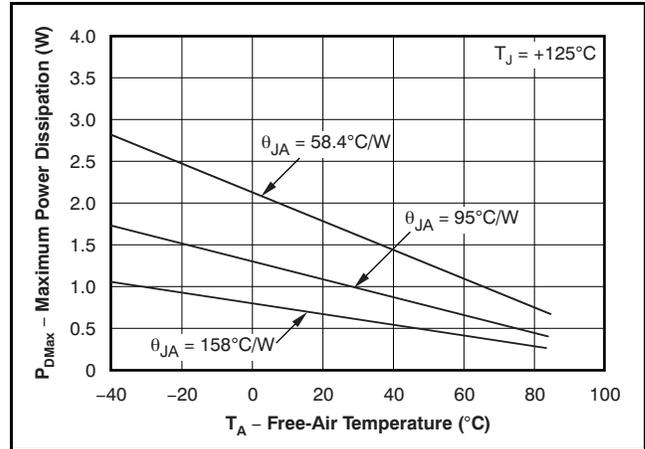
Results shown are with no air flow and PCB size of 3 in x 3 in (76,2 mm x 76,2 mm).
