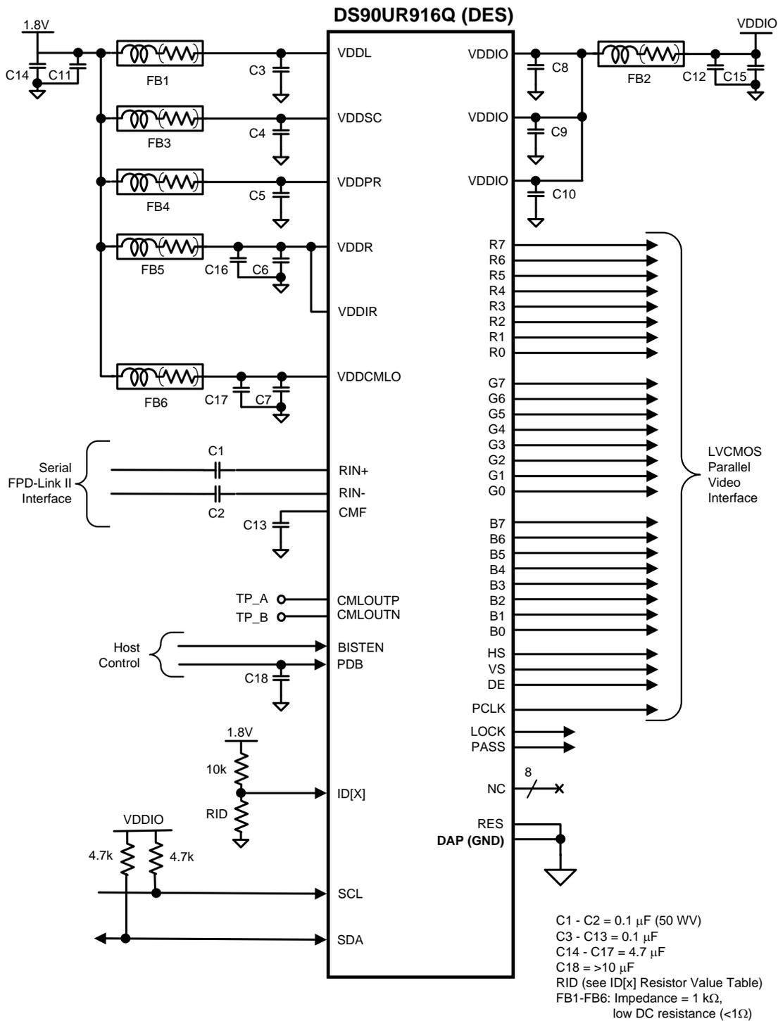
Figure 31. DS90UR916Q Typical Connection Diagram — Pin Control
