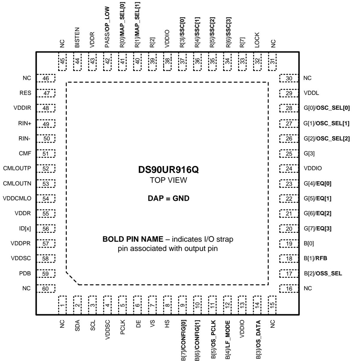
Figure 3. Deserializer - DS90UR916Q — Top View
