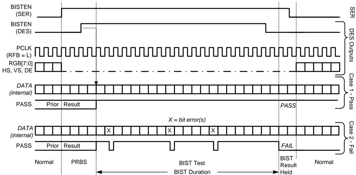
Figure 26. BIST Waveforms
