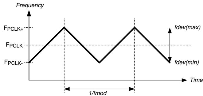
**Figure 19. SSCG Waveform**
