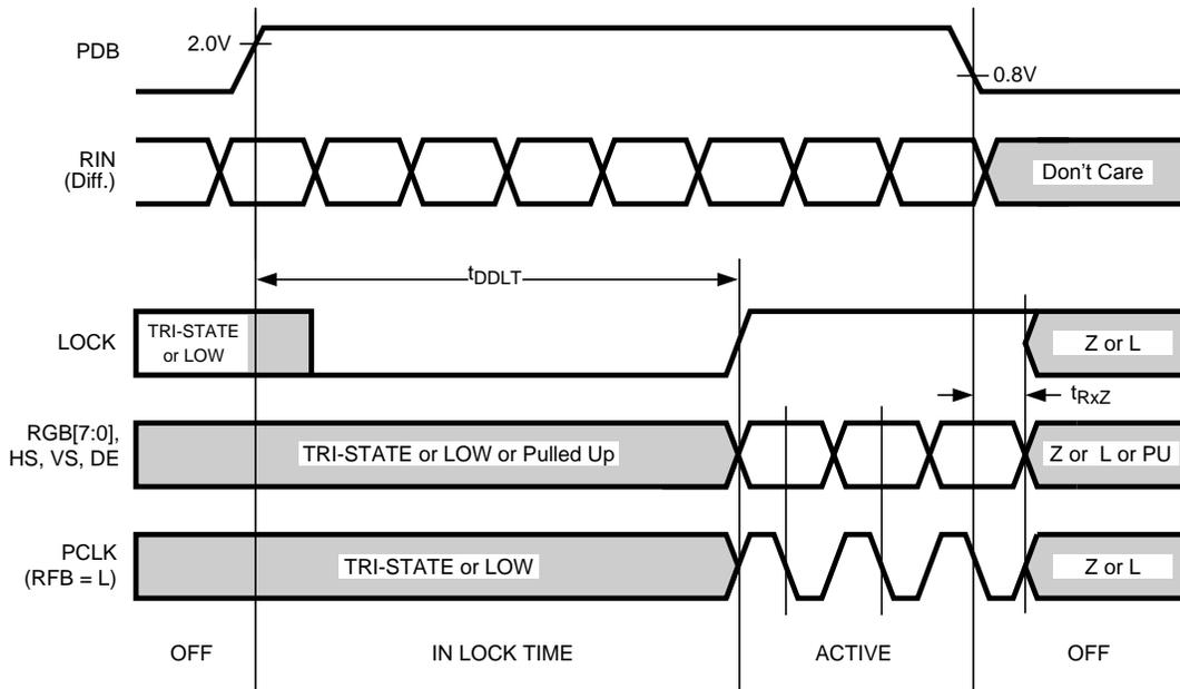
Figure 8. Deserializer PLL Lock Times and PDB TRI-STATE Delay<sup>(1)</sup>
