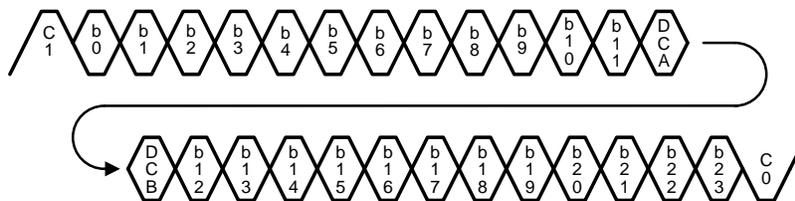
Figure 14. FPD-Link II Serial Stream (905/916)
