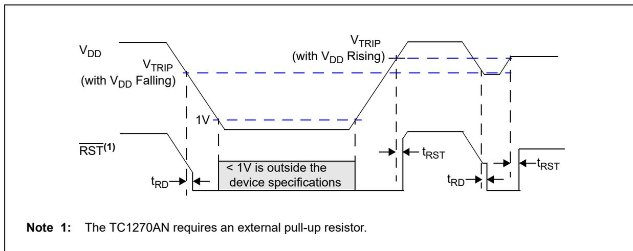
**FIGURE 4-8:**  $\overline{RST}$  Operation as determined by the  $V_{TRIP}$ .
