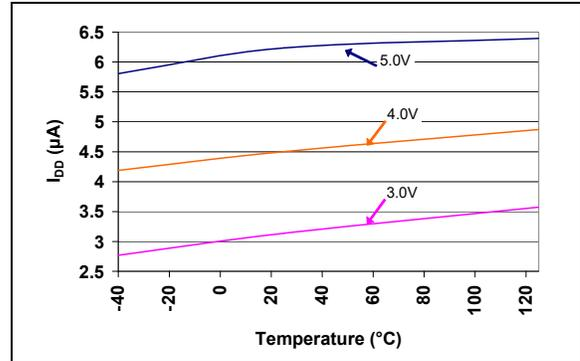
**FIGURE 2-6:**  $I_{DD}$  vs. Temperature (Reset Power-up Timer Active)
