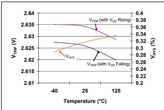
**FIGURE 2-15:**  $V_{TRIP}$  and  $V_{HYS}$  vs. Temperature
