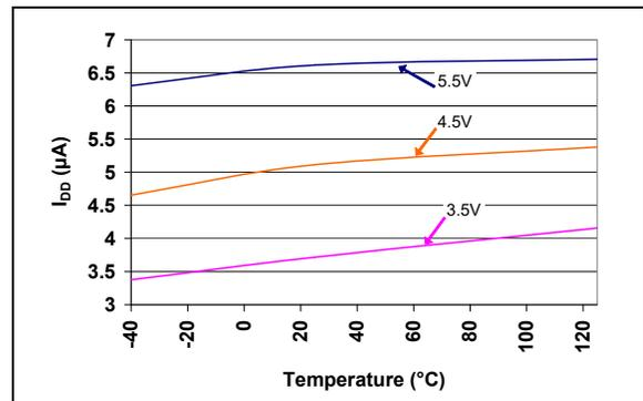
**FIGURE 2-5:**  $I_{DD}$  vs. Temperature (Reset Power-up Timer Active)
