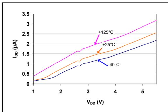
**FIGURE 2-9:**  $I_{DD}$  vs.  $V_{DD}$  (Reset Power-up Timer Inactive)
