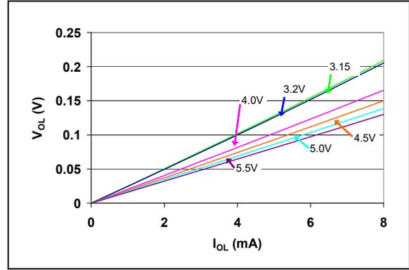
**FIGURE 2-17:**  $V_{OL}$  vs.  $I_{OL}$
