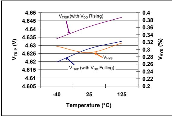
**FIGURE 2-13:**  $V_{TRIP}$  and  $V_{HYS}$  vs. Temperature
