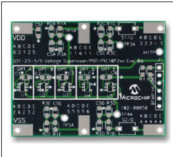
**FIGURE 8-1:** SOT-23-5/6 Voltage Supervisor Evaluation Board (VSUPEV2).
