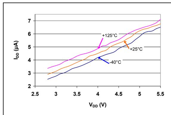
**FIGURE 2-12:**  $I_{DD}$  vs.  $V_{DD}$  (Reset Power-up Timer Active)
