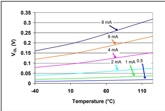
**FIGURE 2-20:**  $V_{OL}$  vs. Temperature
