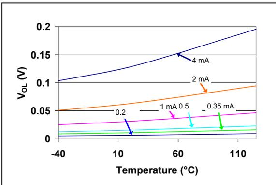
**FIGURE 2-21:**  $V_{OL}$  vs. Temperature
