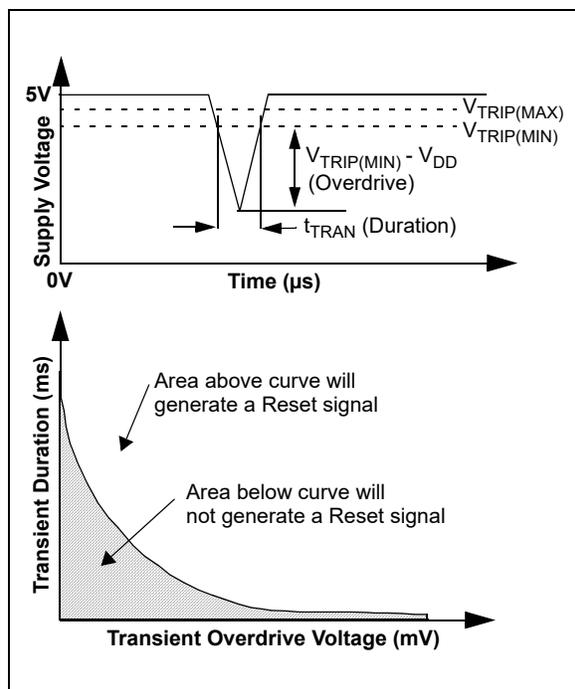
**FIGURE 4-9:** Example of Typical Transient Duration Waveform.
