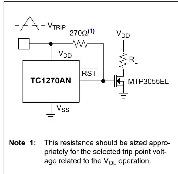
**FIGURE 5-6:** MOSFET Low-Drive Protection.
