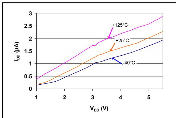
**FIGURE 2-8:**  $I_{DD}$  vs.  $V_{DD}$  (Reset Power-up Timer Inactive)
