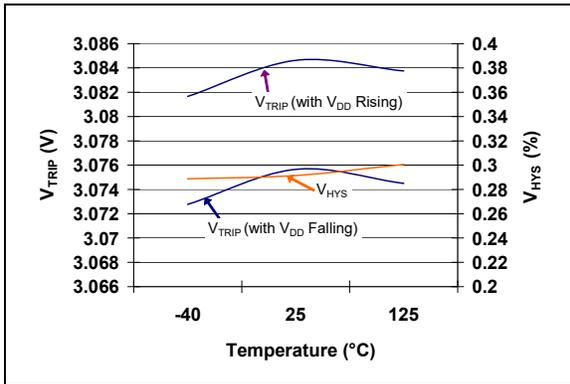
**FIGURE 2-14:**  $V_{TRIP}$  and  $V_{HYS}$  vs. Temperature
