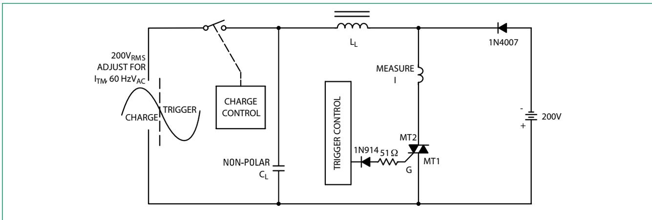
Note: Component values are for verification of rated  $(di/dt)_c$ . See AN1048 for additional information
