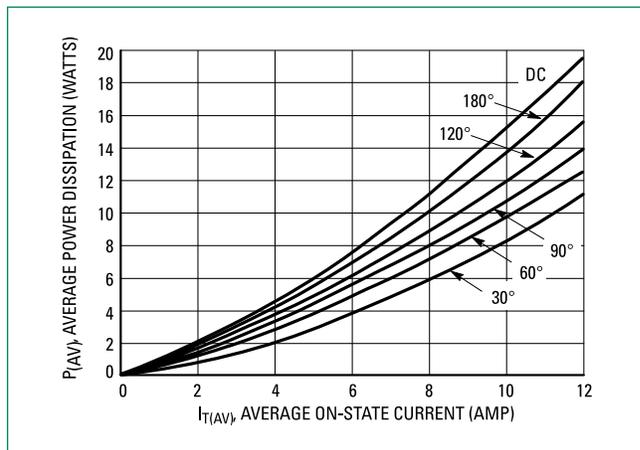
**Figure 3. On-State Characteristics**
