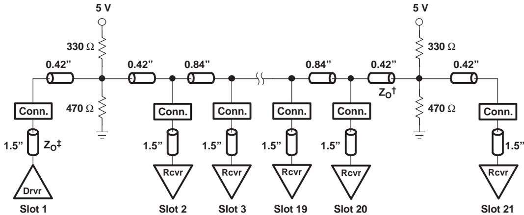
† Unloaded backplane trace natural impedance ( $Z_0$ ) is 45  $\Omega$ . 45  $\Omega$  to 60  $\Omega$  is allowed, with 50  $\Omega$  being ideal.
