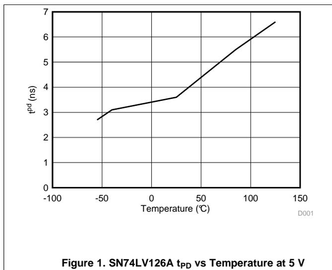
Figure 1. SN74LV126A  $t_{PD}$  vs Temperature at 5 V
