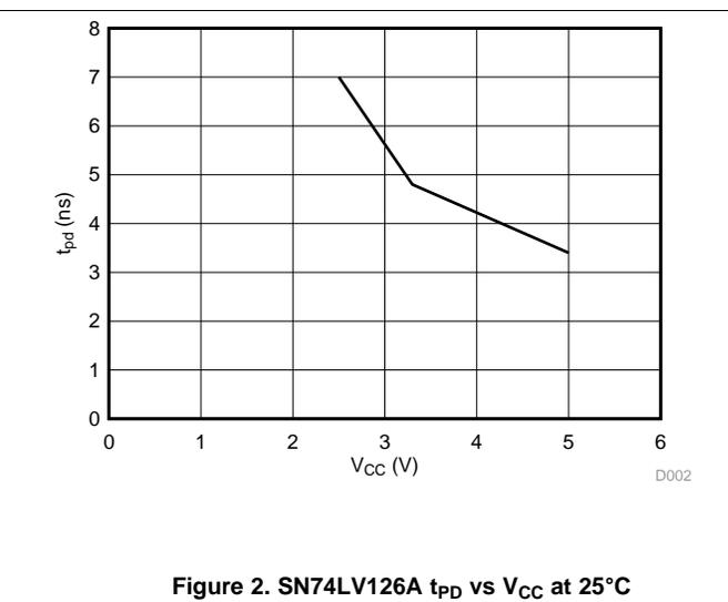
Figure 2. SN74LV126A  $t_{PD}$  vs  $V_{CC}$  at 25°C
