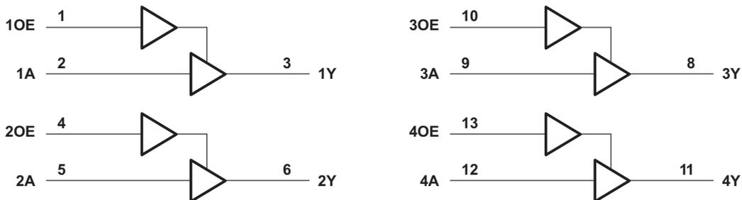
A. Pin numbers shown are for the D, DB, DGV, J, N, NS, PW, and W packages.
