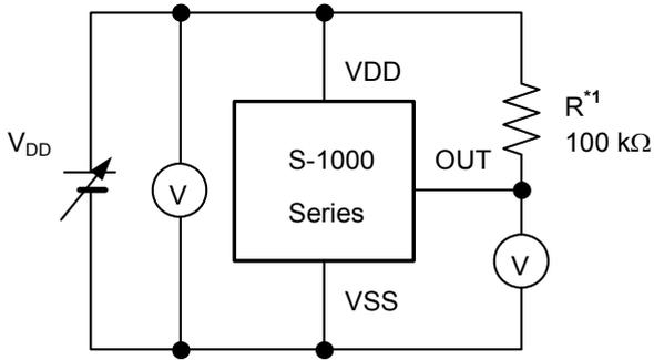
1. R is unnecessary for CMOS output products.
