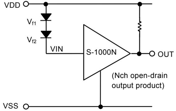
$$\text{Detection voltage} = V_{f1} + V_{f2} + (-V_{DET})$$
