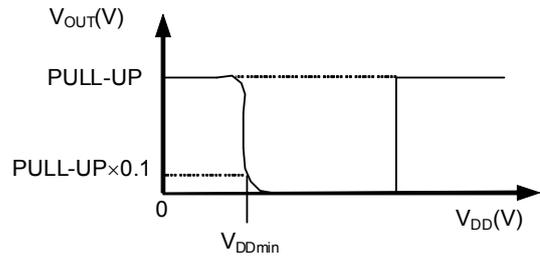
**Remark**  $V_{DDmin}$  is defined by the  $V_{DD}$  voltage at which  $V_{OUT}$  goes below 10% of pull-up voltage when the  $V_{DD}$  increase from 0 V.
