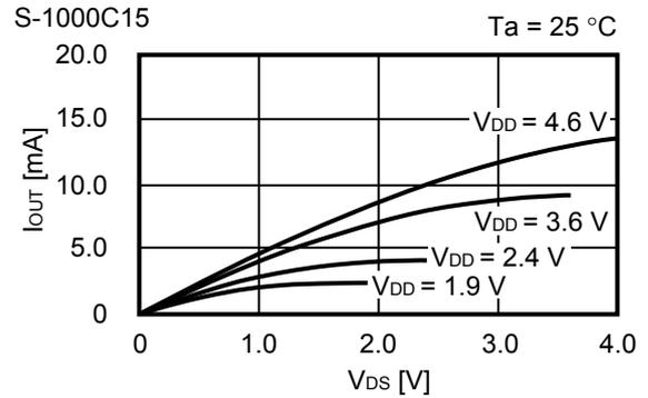
7. Nch transistor output current ( $I_{OUT}$ )
