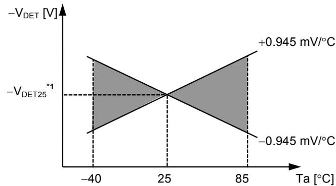
\*1. □-V<sub>DET25</sub> is an actual detection voltage value at 25°C.
