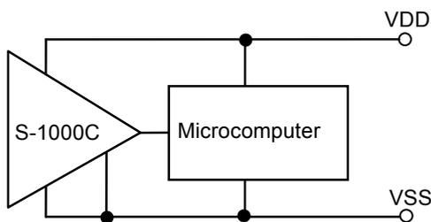
**Figure 24** Reset circuit example(S-1000C)
