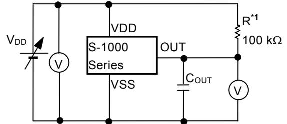
\*1. R is unnecessary for CMOS output products.
