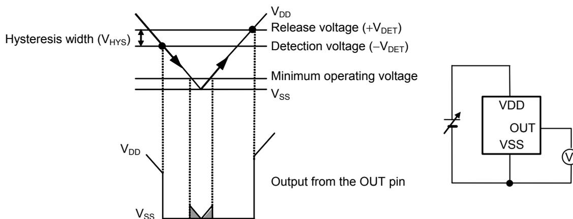
**Remark** For values of  $V_{DD}$  less than minimum operating voltage, values of OUT terminal output is free in the shaded region.
