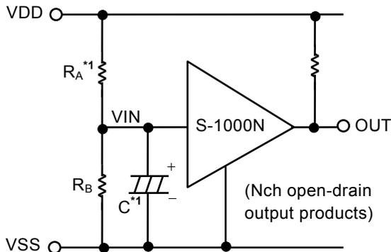
$$\text{Detection voltage} = \frac{R_A + R_B}{R_B} \cdot -V_{DET}$$
