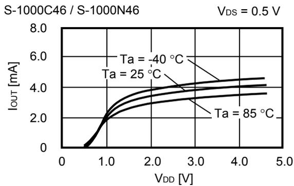
8. Pch transistor output current ( $I_{OUT}$ )
