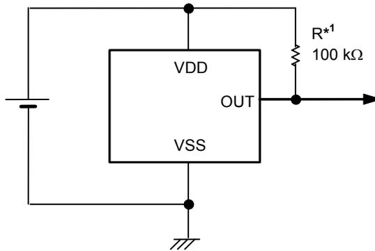
\*1. R is unnecessary for CMOS output products.
