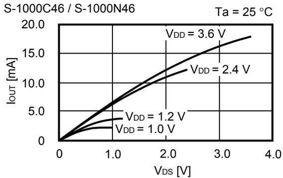
6. Pch transistor output current ( $I_{OUT}$ ) –  $V_{DS}$
