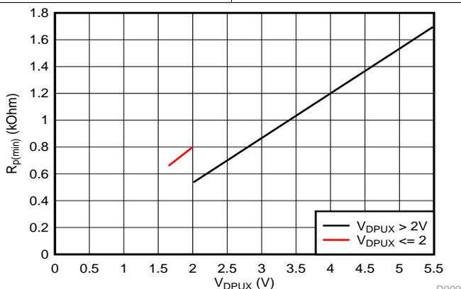
$V_{OL} = 0.2 \cdot V_{DPUX}$ ,  $I_{OL} = 2 \text{ mA}$  when  $V_{DPUX} \leq 2 \text{ V}$
