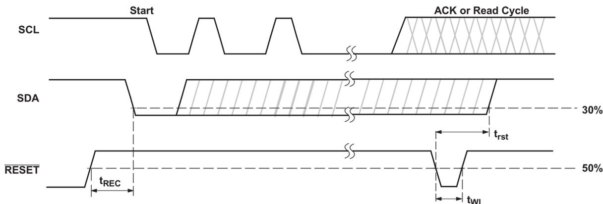
Figure 2. Reset Timing
