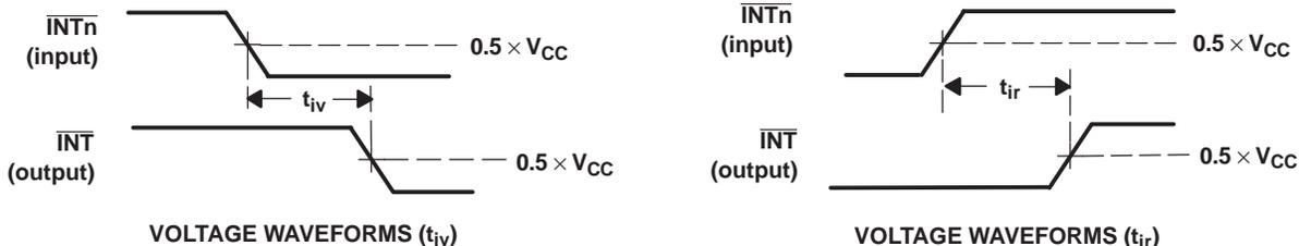
VOLTAGE WAVEFORMS ( $t_{iv}$ )
