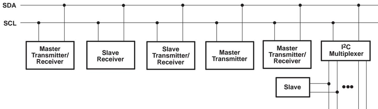
Figure 6. System Configuration
