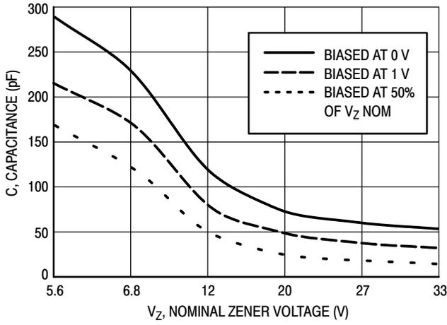
Figure 1. Typical Capacitance
