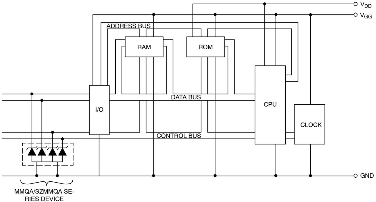
Figure 10. Microprocessor Protection
