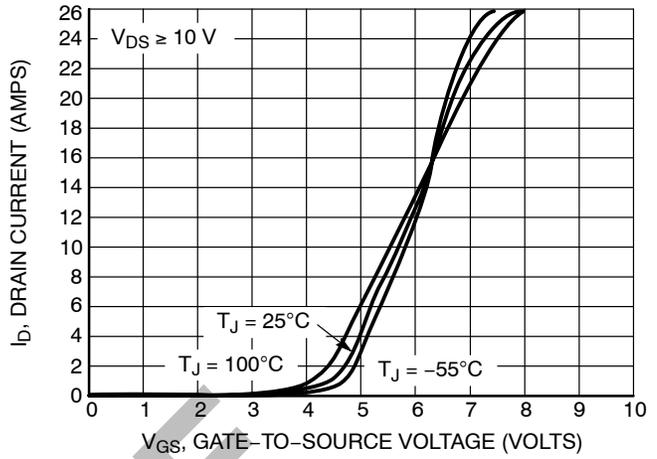
Figure 2. Transfer Characteristics
