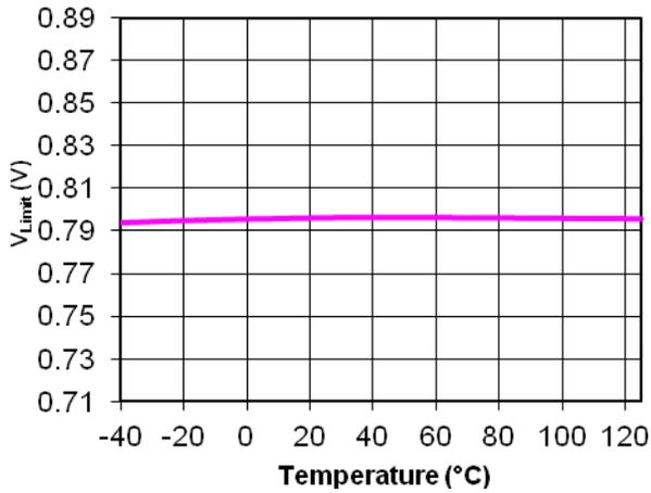
Figure 9. V<sub>Limit</sub> vs. Junction Temperature
