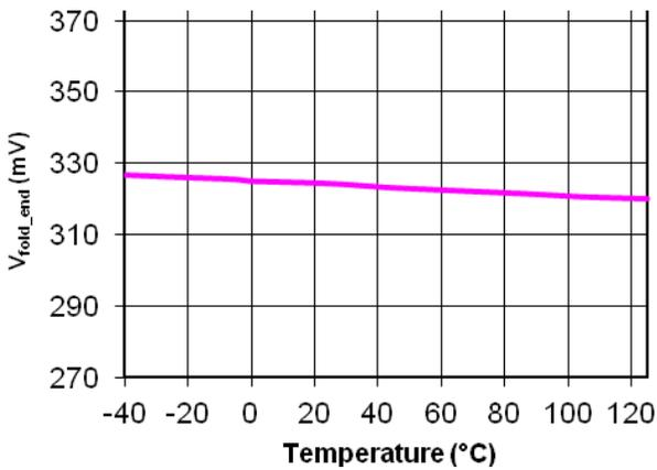
Figure 19. V<sub>fold\_end</sub> vs. Junction Temperature
