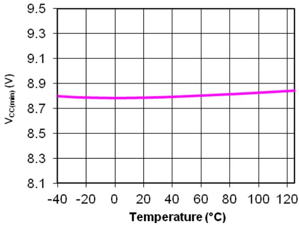
Figure 11. V<sub>CC(min)</sub> vs. Junction Temperature
