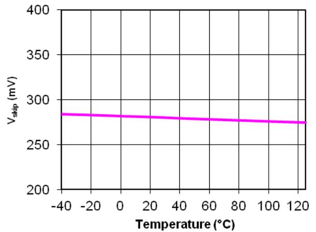
Figure 20. V<sub>skip</sub> vs. Junction Temperature
