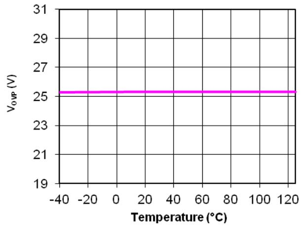
Figure 24. V<sub>OVP</sub> vs. Junction Temperature
