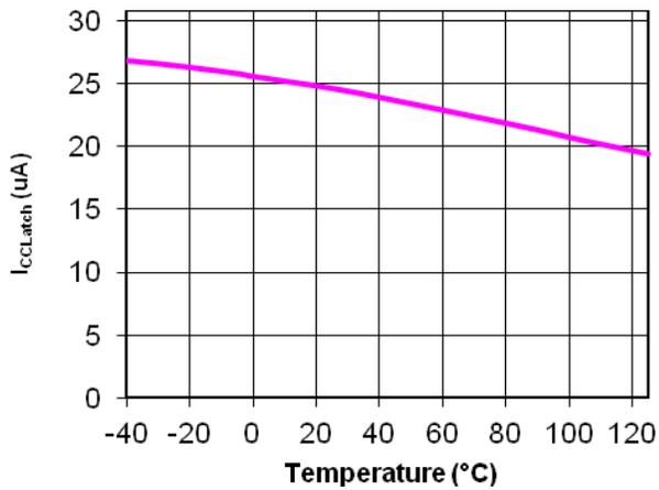
Figure 13. I<sub>CCLatch</sub> vs. Junction Temperature
