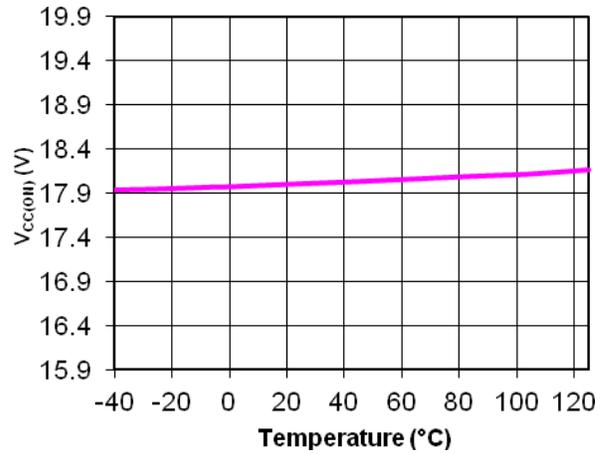
Figure 10. V<sub>CC(ON)</sub> vs. Junction Temperature
