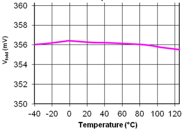
Figure 17. V<sub>fold</sub> vs. Junction Temperature
