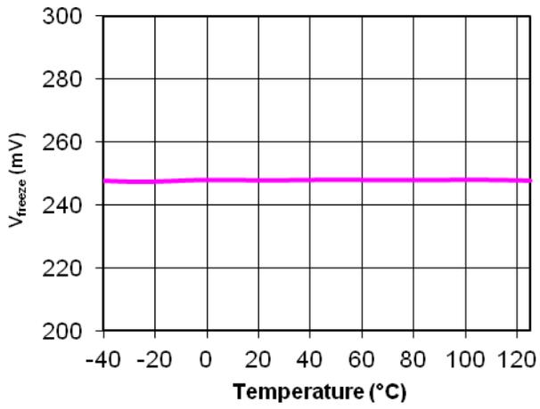
Figure 21. V<sub>freeze</sub> vs. Junction Temperature
