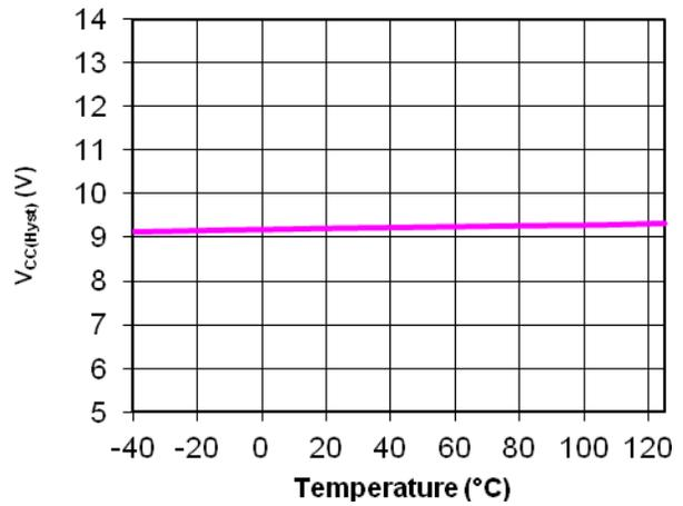
Figure 12. V<sub>CC(Hyst)</sub> vs. Junction Temperature
