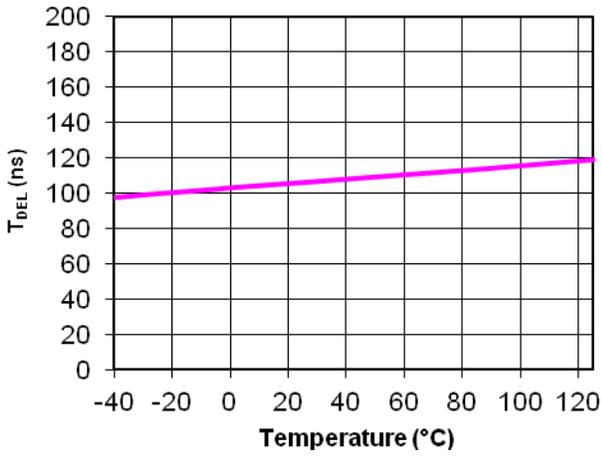
Figure 15. T<sub>DEL</sub> vs. Junction Temperature
