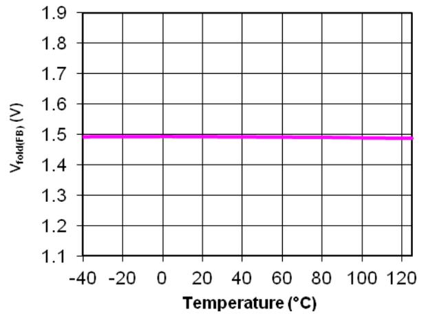
Figure 18. V<sub>fold(FB)</sub> vs. Junction Temperature
