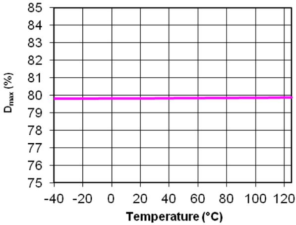
Figure 3. D<sub>max</sub> vs. Junction Temperature
