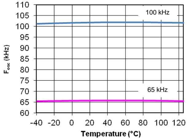
Figure 4. F<sub>osc</sub> vs. Junction Temperature
