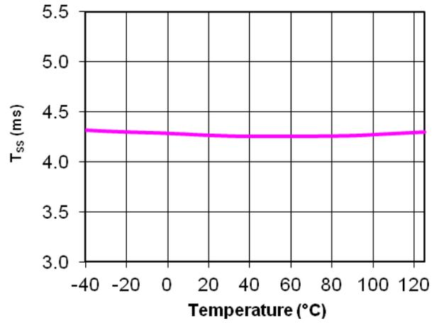
Figure 16. T<sub>SS</sub> vs. Junction Temperature
