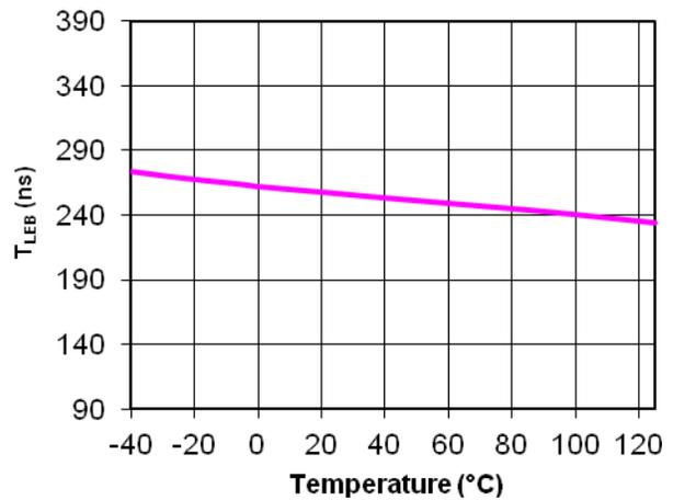
Figure 14. T<sub>LEB</sub> vs. Junction Temperature
