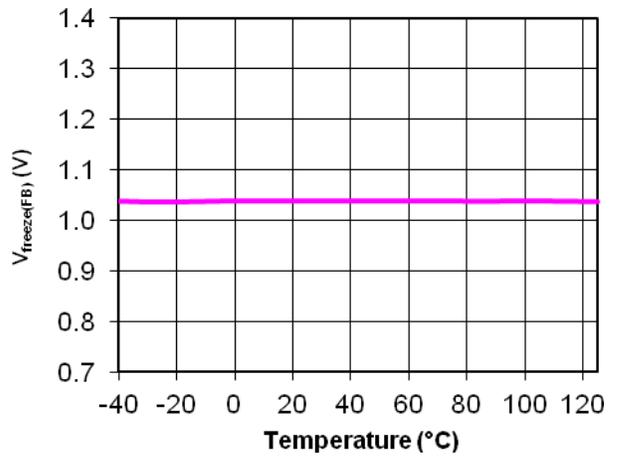
Figure 22. V<sub>freeze(FB)</sub> vs. Junction Temperature
