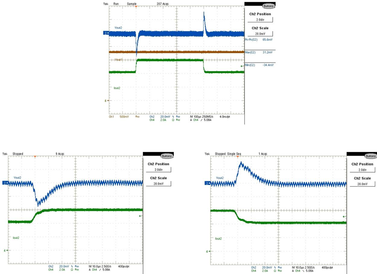
Figure 39:  $V_{out2}$  Transient Response, 4.2A to 6A step at  $2.5A/\mu Sec$
