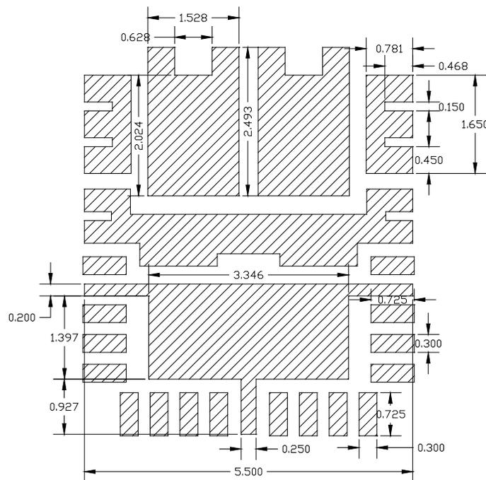
Figure 46: SMD Pad Sizes Detail 1 (Dimensions in mm)
