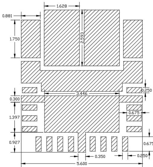
Figure 43: PCB Pad Sizes Detail 1
