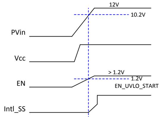
Figure 4: Normal Startup: IR3892 Channel starts when P<sub>Vin</sub> reaches 10.2V by connecting EN to P<sub>Vin</sub> using a resistor divider.
