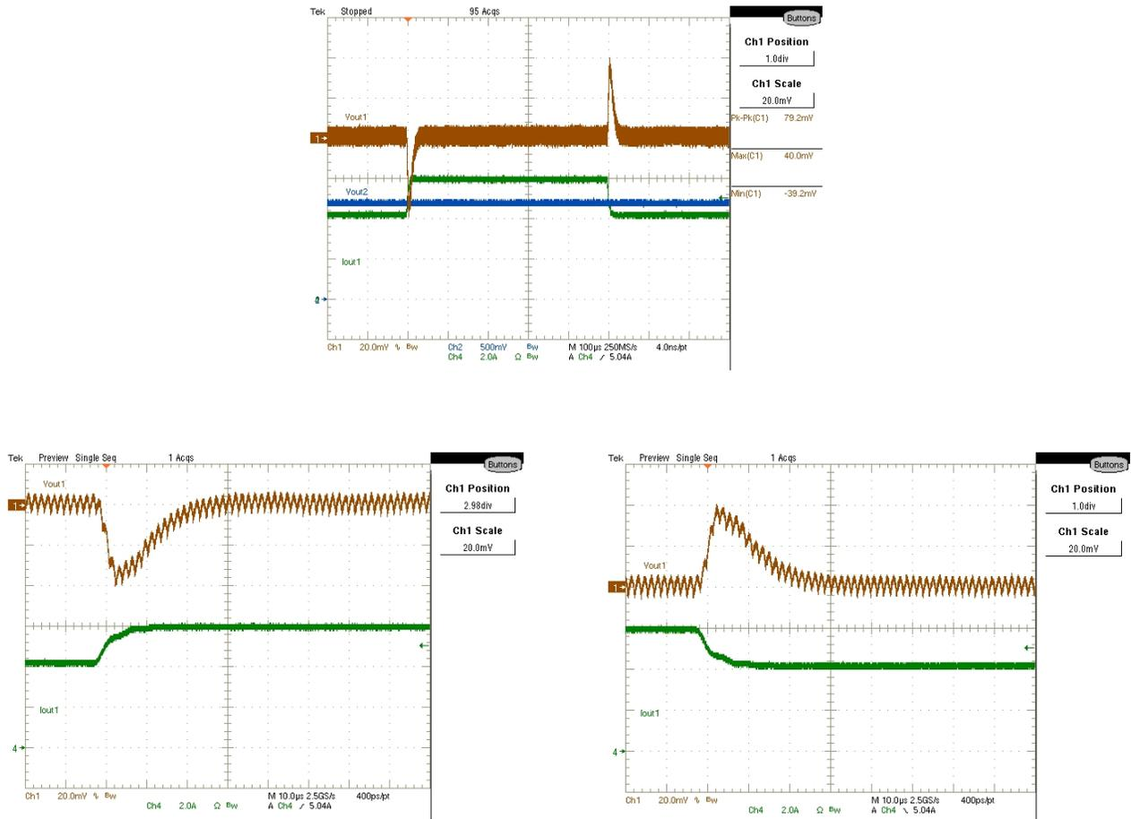
Figure 38: Vout1 Transient Response, 4.2A to 6A step at 2.5A/μSec
