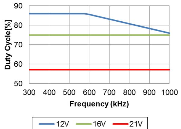
Figure 22: Maximum Duty Cycle vs. Switching Frequency
