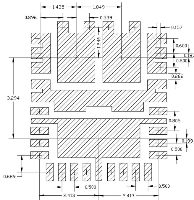
Figure 48: SMD Pad Spacing (Dimensions in mm)
