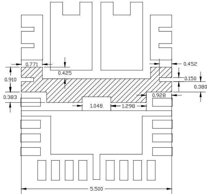
Figure 47: SMD Pad Sizes Detail 2 (Dimensions in mm)
