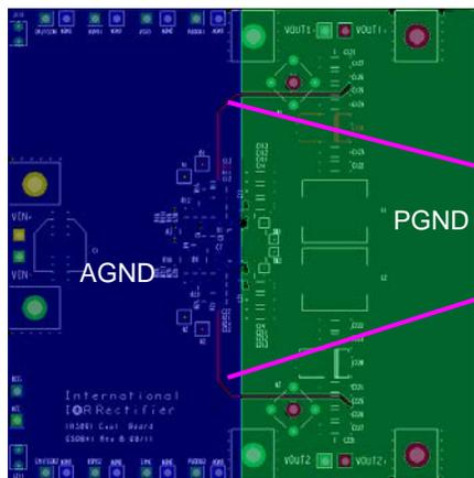
Feedback and Vsns trace routing should be kept away from noise sources
