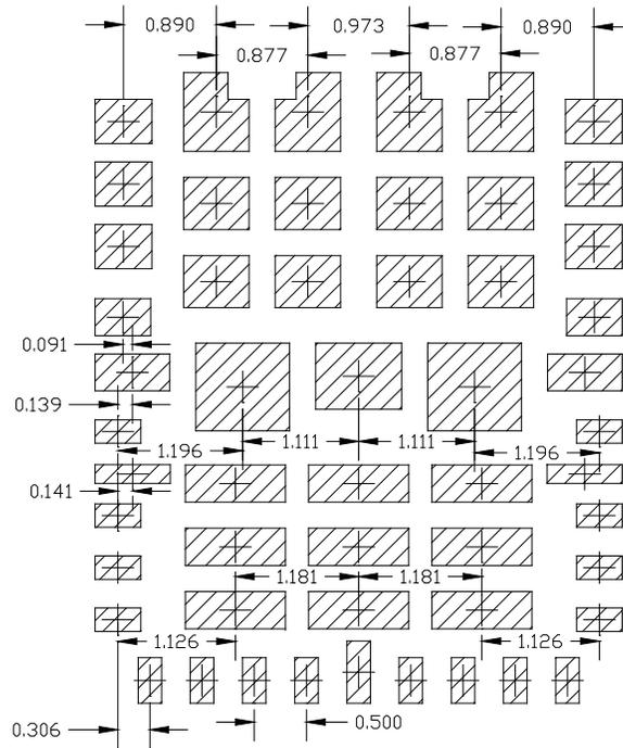
Figure 50: Stencil Pad Spacing Detail 1 (Dimensions in mm)
