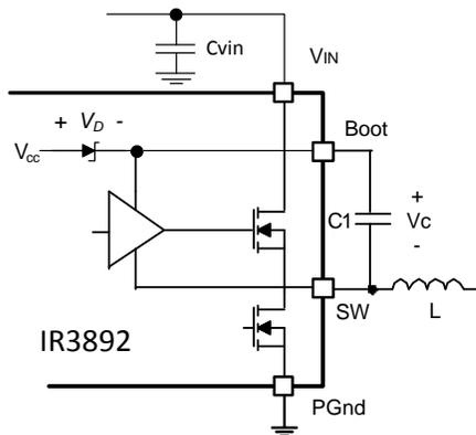
Figure 25: Bootstrap circuit to generate  $V_c$  voltage
