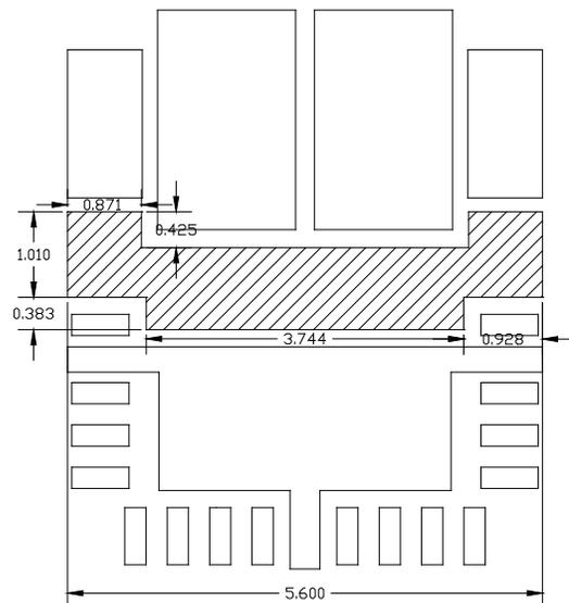
Figure 44: PCB Pad Sizes Detail 2
