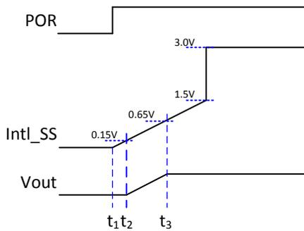
Figure 9: Theoretical operation waveforms during soft-start (non-sequencing)
