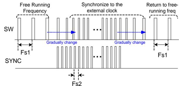
Figure 10: Timing diagram for synchronization to an external clock ( $F_{s1} > F_{s2}$  or  $F_{s1} < F_{s2}$ )
