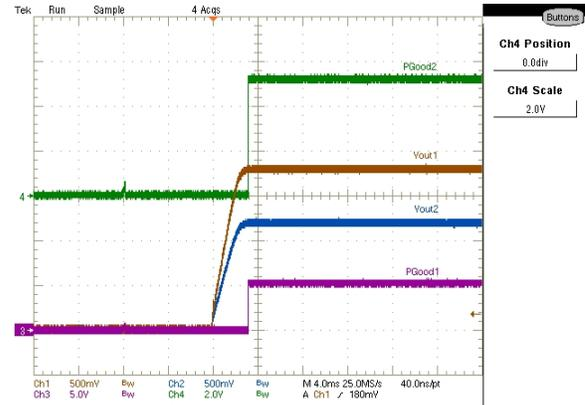
Figure 33: PGood signals at Startup with full load
