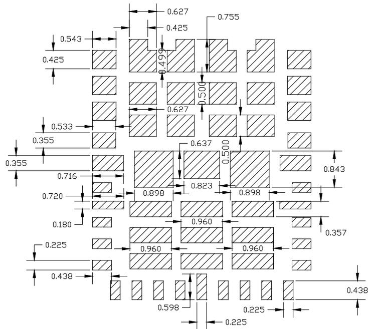
Figure 49: Stencil Pad Sizes (Dimensions in mm)
