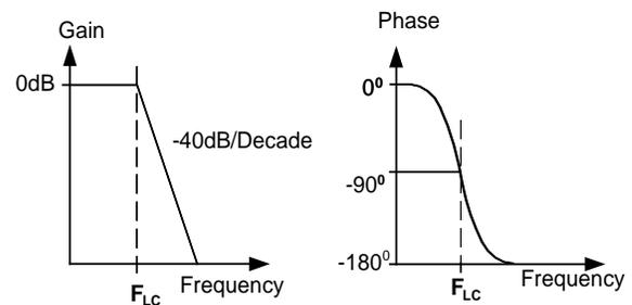
Figure 26: Gain and Phase of LC filter
