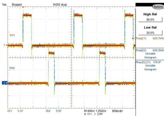
Figure 36: Inductor Switch Nodes at full load
