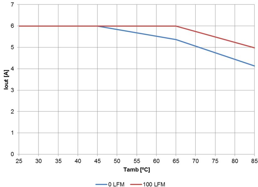
$V_{in}=P_{Vin}=12V$ ,  $V_{out1} = 3.3V$ ,  $V_{out2}=1.8V$ ,  $I_{out1} = I_{out2}$ ,  $V_{CC}=\text{internal LDO (5.3V)}$ ,  $F_s = 600kHz$
