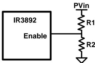
Figure 23: Using Enable pin for UVLO implementation
