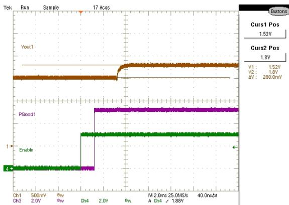
Figure 34: Channel 1 Startup with Pre-Bias, 1.52V
