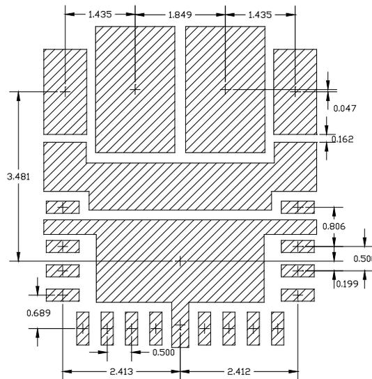
Figure 45: PCB Metal Pad Spacing (Dimensions in mm)
