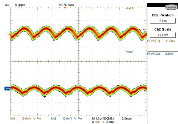
Figure 37: Output Voltage Ripples at full load
