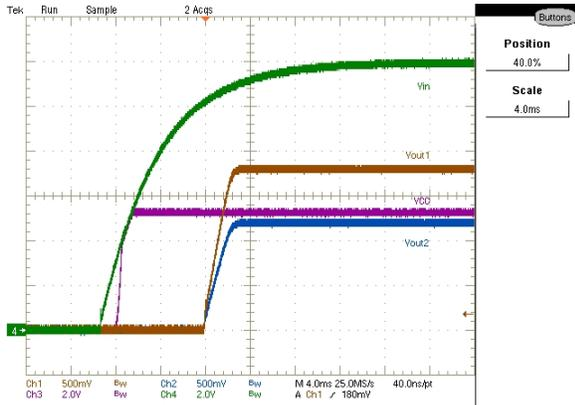
Figure 32: Startup with full load
