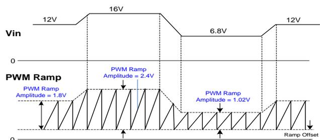
Figure 12: Timing diagram for Feed Forward (F.F.) Function
