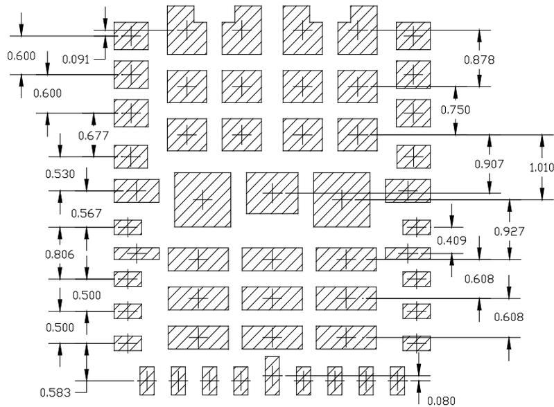
Figure 51: Stencil Pad Spacing Detail 2 (Dimensions in mm)
