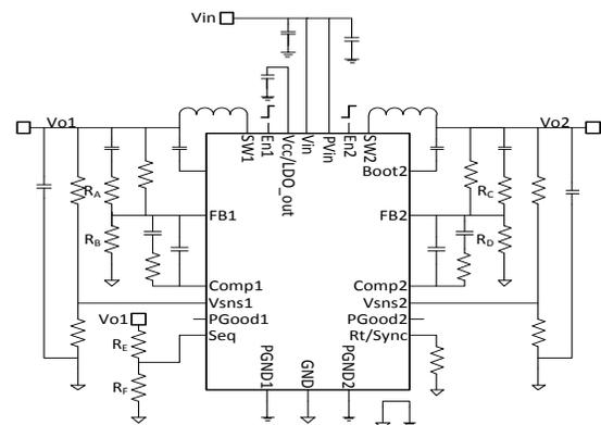
Figure 18: Application Circuit for Simultaneous and Ratiometric Sequencing
