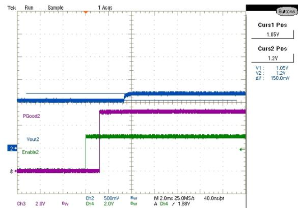
Figure 35: Channel 2 Startup with Pre-Bias, 1.05V
