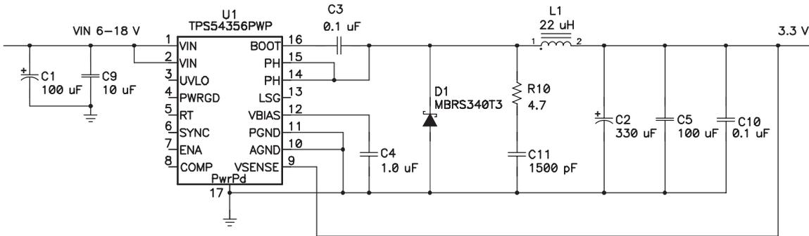
Figure 26. 3.3-V Power Supply With Schottky Diode
