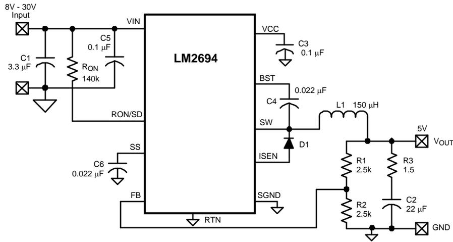
**Figure 14. Example Circuit**
