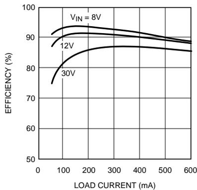
**Figure 15. Efficiency vs Load Current and V<sub>IN</sub>**
