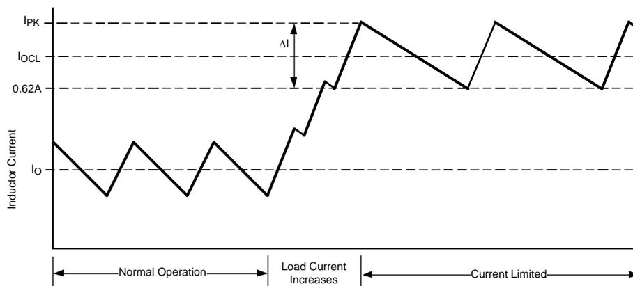
**Figure 12. Inductor Current - Current Limit Operation**
