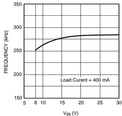
**Figure 16. Frequency vs V<sub>IN</sub>**
