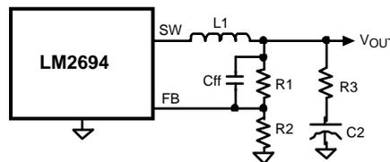
Figure 18. Low Output Ripple Using a Feedforward Capacitor
