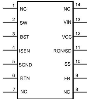
**Figure 1. 14-Lead TSSOP Package**
