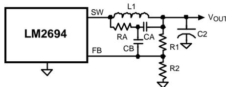
Figure 19. Minimum Output Ripple Using Ripple Injection
