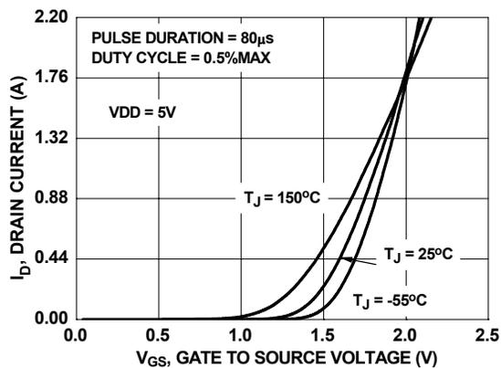
Figure 5. Transfer Characteristics
