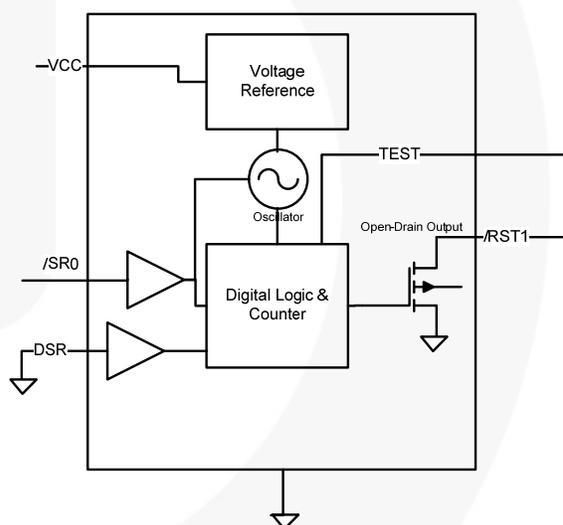
Figure 1. Block Diagram
